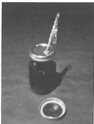
Figure 3. Pierced canning jar lid forms micro fermentation lock.
